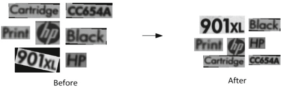
Fig. 3. Illustrative examples of image correction results obtained through applying the rotation and skew correction algorithm. The algorithm improves the blurry images for OCR.
